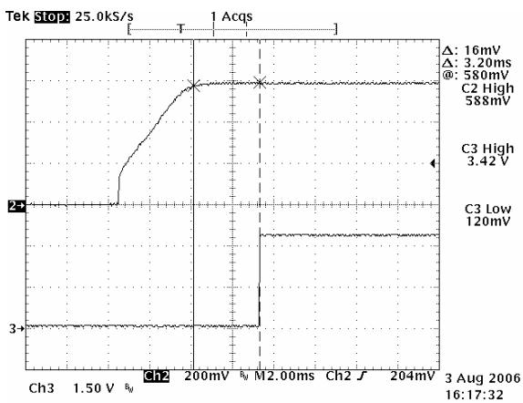
**Figure 51:** Power Good delay time by on/off
