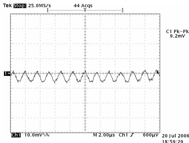
**Figure 5:** Output Ripple & Noise
