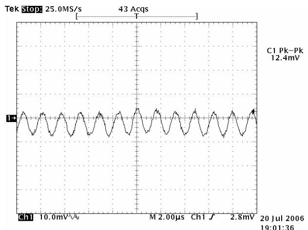
**Figure 6:** Output Ripple & Noise
