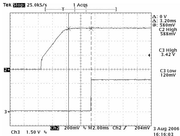
**Figure 49:** Power Good delay time by on/off
