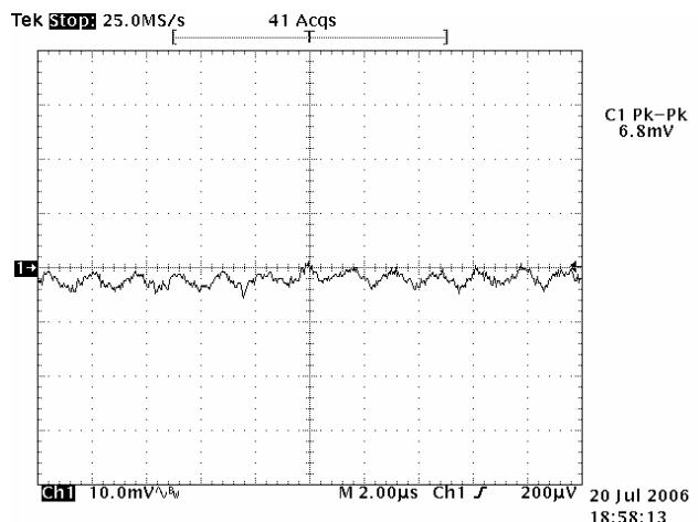
**Figure 4:** Output Ripple & Noise
