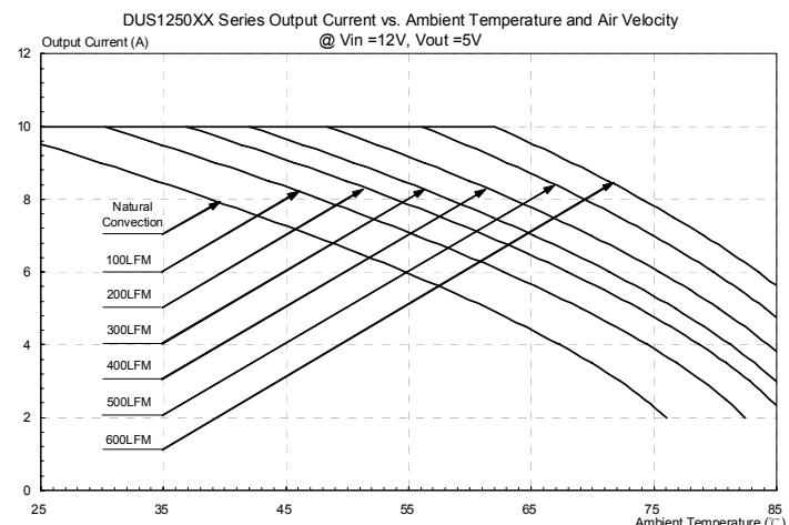
**Figure 59:** Output current vs. ambient temperature and air velocity
