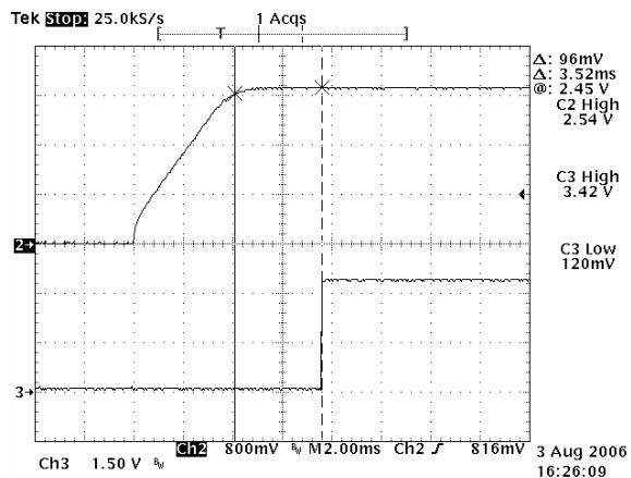
**Figure 50:** Power Good delay time by on/off
