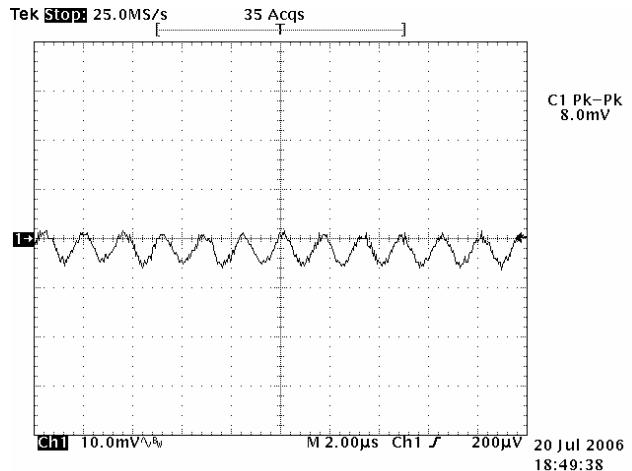
**Figure 2:** Output Ripple & Noise
