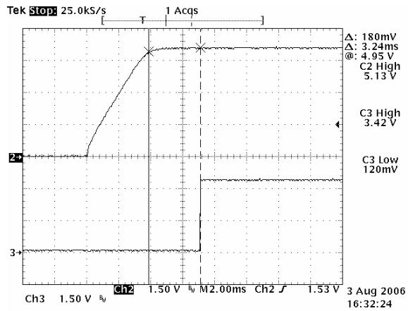
**Figure 54:** Power Good delay time by on/off
