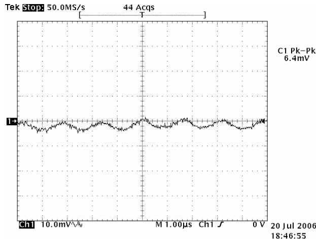
**Figure 1:** Output Ripple & Noise
