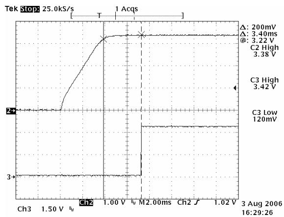
**Figure 52:** Power Good delay time by on/off
