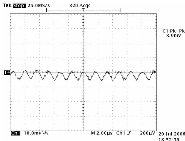
**Figure 3:** Output Ripple & Noise
