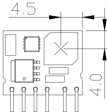
**Figure 58:** Hot spot temperature measured point
