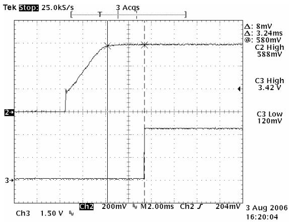
**Figure 53:** Power Good delay time by on/off
