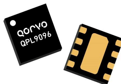
8 Pin 2X2 mm DFN Package
