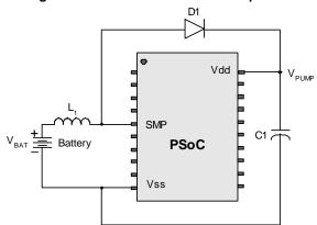
Figure 12. Basic Switch Mode Pump Circuit
