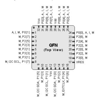
Figure 7. CY8C21634 32-pin PSoC Device
