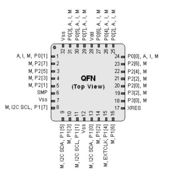
Figure 8. CY8C21434 32-pin Sawn PSoC Device Sawn
