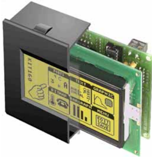
EA KIT160-6LEDTP Dimension 102 x 80 x 36mm Viewing area 70 x 36 mm
