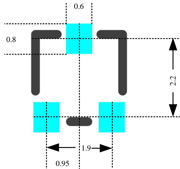
Figure 16. AH9247 Layout Pattern Mechanical Dimensions (Unit: mm)
