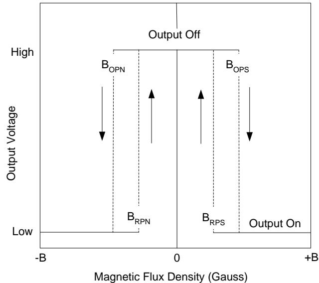
Figure 4. Output Voltage vs. Magnetic Flux Density
