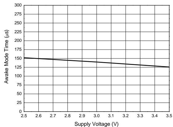
Figure 11. Awake Mode Time vs. Supply Voltage
