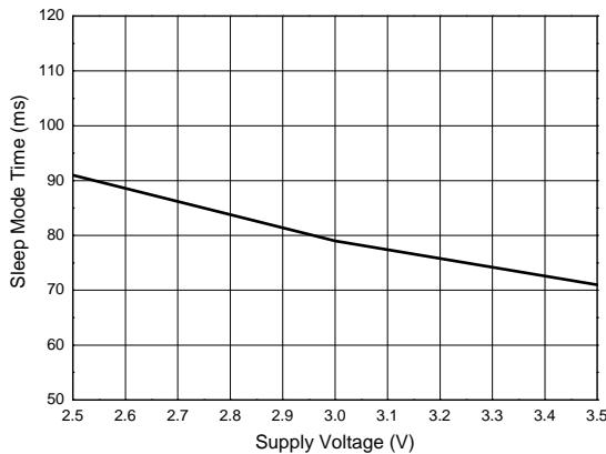
Figure 12. Sleep Mode Time vs. Supply Voltage
