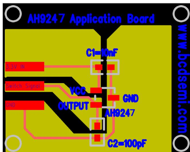
Figure 15. Typical Layout Pattern of AH9247 (Note 11)
