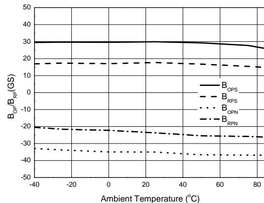
Figure 9.  $B_{OP}/B_{RP}$  vs. Ambient Temperature
