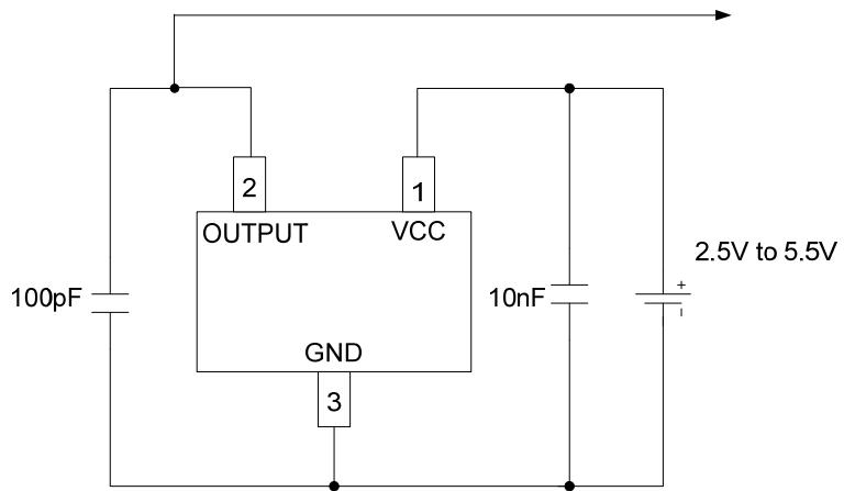
Figure 14. Typical Application Circuit of AH9247
