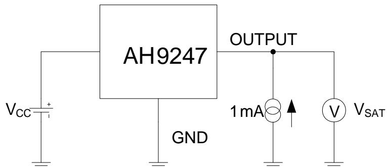
Figure 6. Output Saturation Voltage (Note 7, Note 8)
