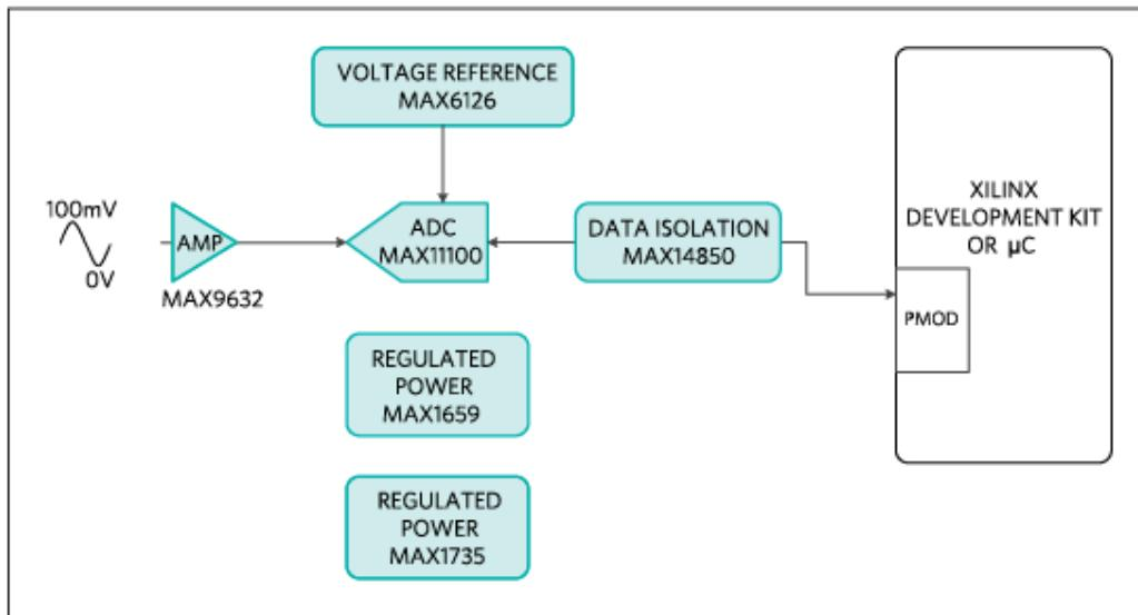
Figure 1. The Fremont subsystem design block diagram.
