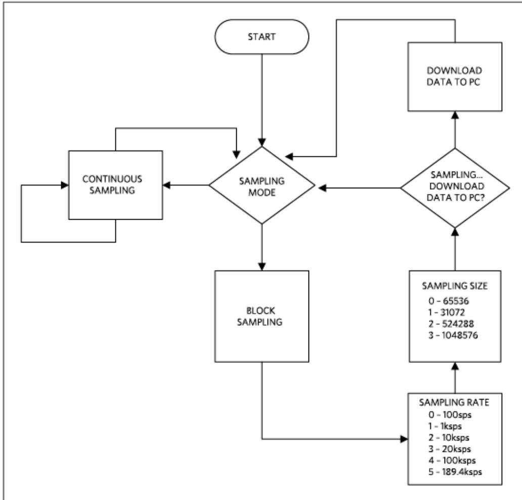
Figure 2b. The Fremont firmware flowchart ZedBoard platform.
