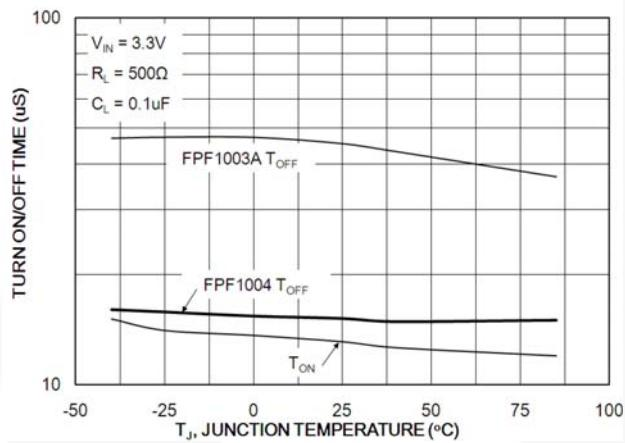
Figure 14. t<sub>ON</sub>/t<sub>OFF</sub> vs. Temperature
