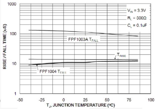
Figure 15. t<sub>R</sub>/t<sub>F</sub> vs. Temperature
