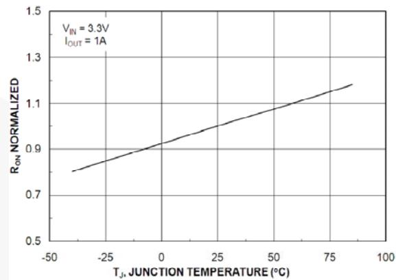
Figure 13. R<sub>ON</sub> vs. Temperature
