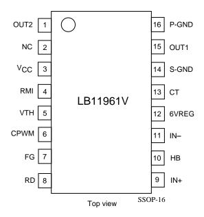
P-GND : Motor system ground S-GND : Control system ground
