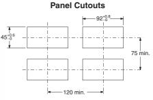
Note: The values above are recommended values. Do not group-mount the meters at intervals less than the recommended ones.
