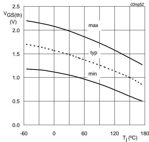
$I_D = 1 \text{ mA}; V_{DS} = V_{GS}$
