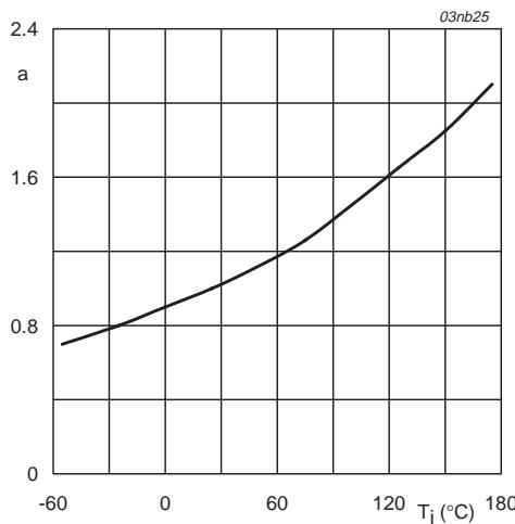
$$a = \frac{R_{DSon}}{R_{DSon}(25^\circ\text{C})}$$
