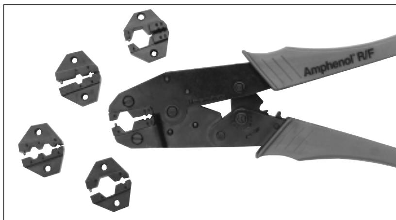
The Amphenol ECONOHEX hand crimp tool is similar in features and application to the TRIHEX crimp tools. However, the ECONOHEX provides the additional feature of die set insertion and removal such that the purchase of the ECONOHEX tool handle and some or all of the four die sets will allow the user to terminate most popular RG coaxial cables as well as Twinaxial cable for IBM system 3X networks.
