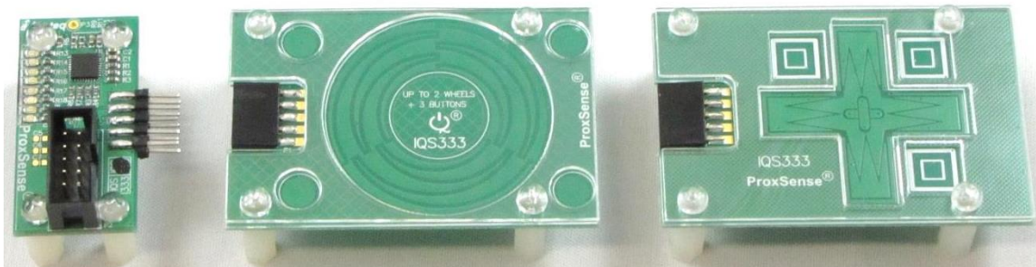
Figure 1.1 Connection board (left), wheel module board (middle) and cross module board (right)
