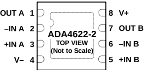
Figure 4. 8-Lead LFCSP Pin Configuration
