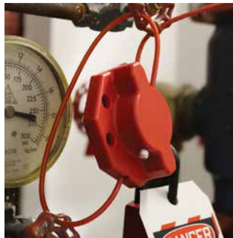
Turn the hasp halves to cinch cable.
