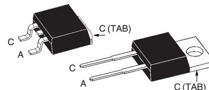
A = Anode, C = Cathode, TAB = Cathode
