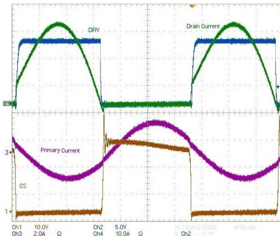
Figure 37. Waveforms from SR System Using MOSFET in TO220 Package with Parasitic Inductance Compensation – SR MOSFET Channel Conduction Time Optimized
