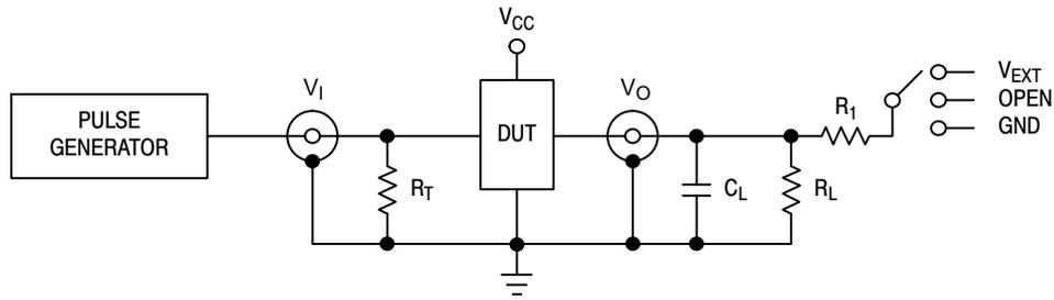
$C_L$  includes jig and probe capacitance
