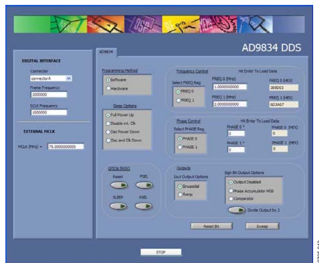
Figure 40. AD9834 Evaluation Software
