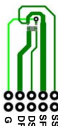
b. 145\text{ }^\circ\text{C}/\text{W} when mounted on a minimum pad of 2 oz copper.
