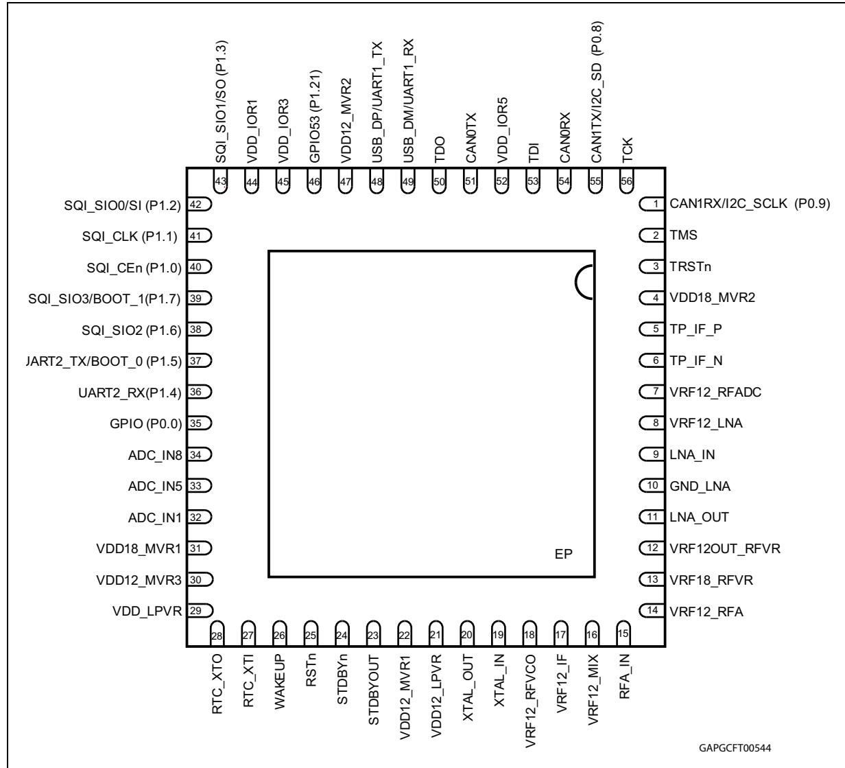
Figure 3. VFQFPN56 connection diagram - no CAN (bottom view)
