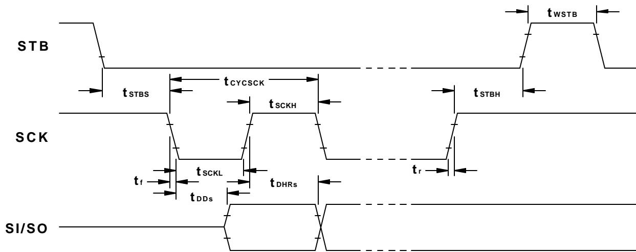
**Figure 8.** Synchronous Serial Interface Read Cycle Timing
