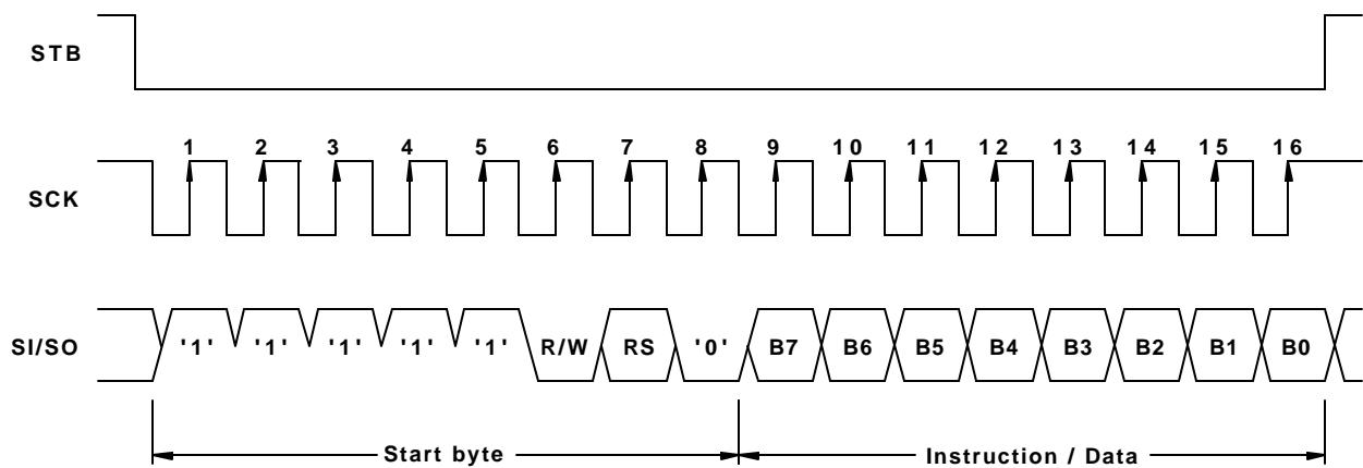
**Figure 11.** Typical Synchronous Serial Interface Write Cycle
