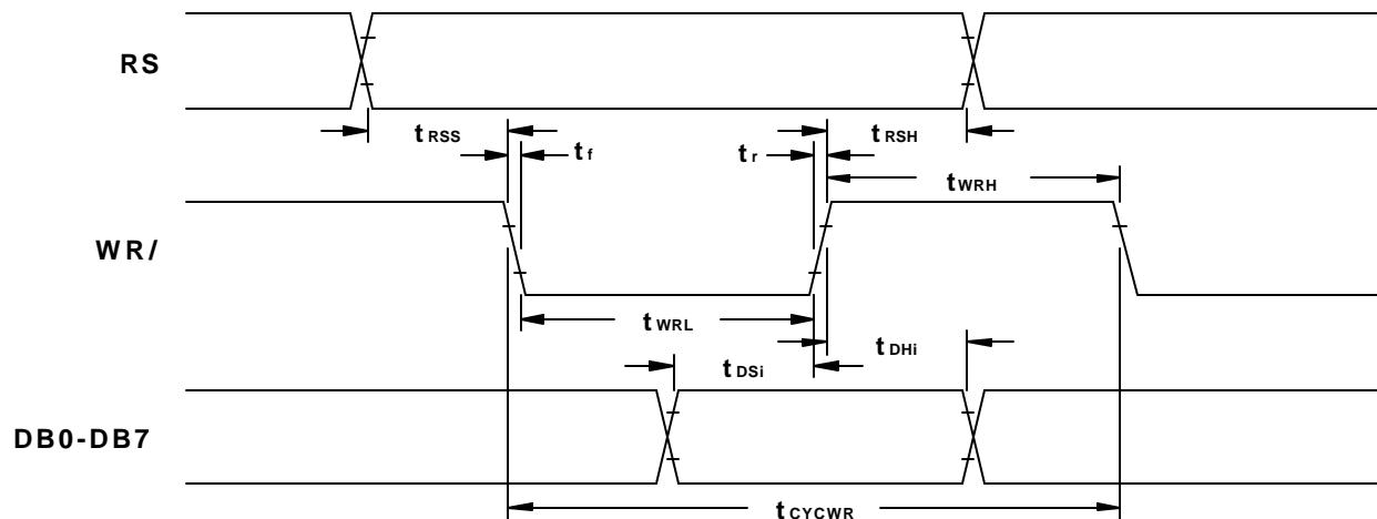
**Figure 5.** Intel I80-Type Parallel Interface Write Cycle Timing
