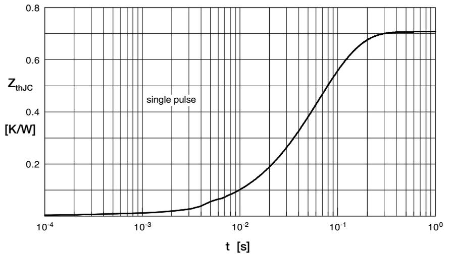
Fig. 2 Typ. transient thermal impedance junction to case
