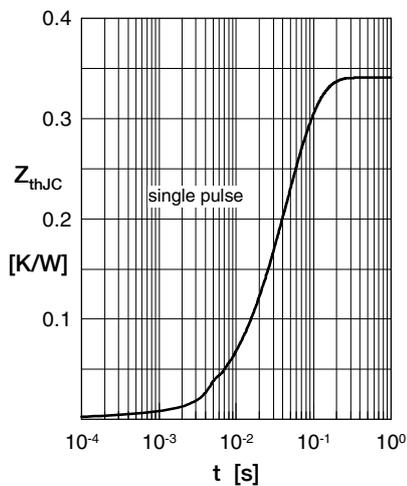
Fig. 12 Typical transient thermal impedance
