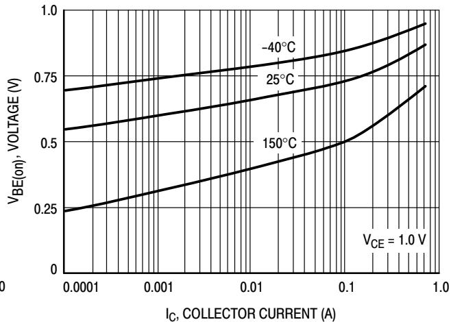
**Figure 8.  $V_{BE(on)}$  Voltage**
