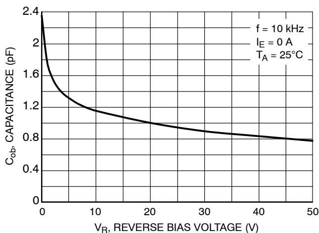
Figure 14. Output Capacitance
