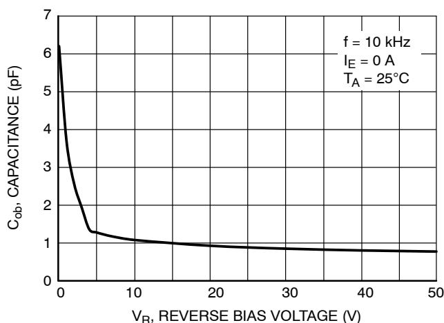
Figure 9. Output Capacitance
