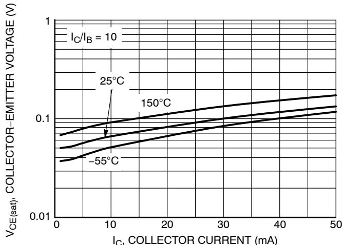
Figure 17.  $V_{CE(\text{sat})}$  vs.  $I_C$
