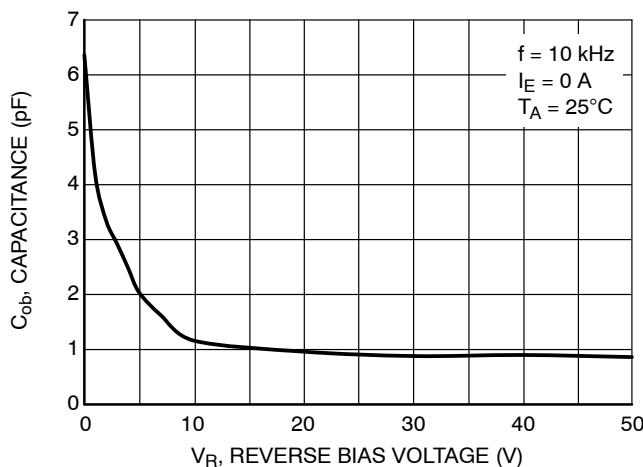
Figure 19. Output Capacitance
