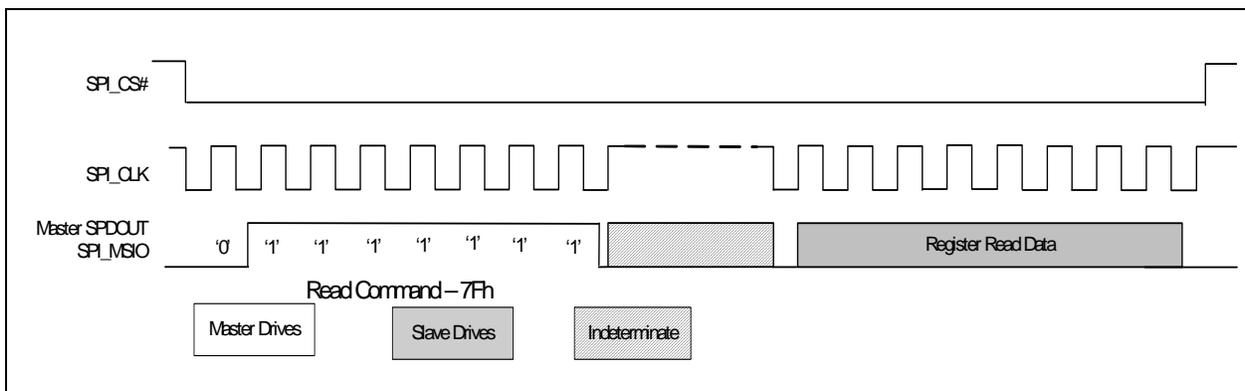
Figure 3.12 SPI Read Data Command - Bi-directional Mode
