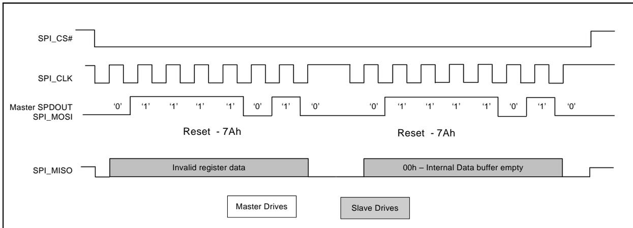
Figure 3.4 SPI Reset Interface Command - Normal Mode
