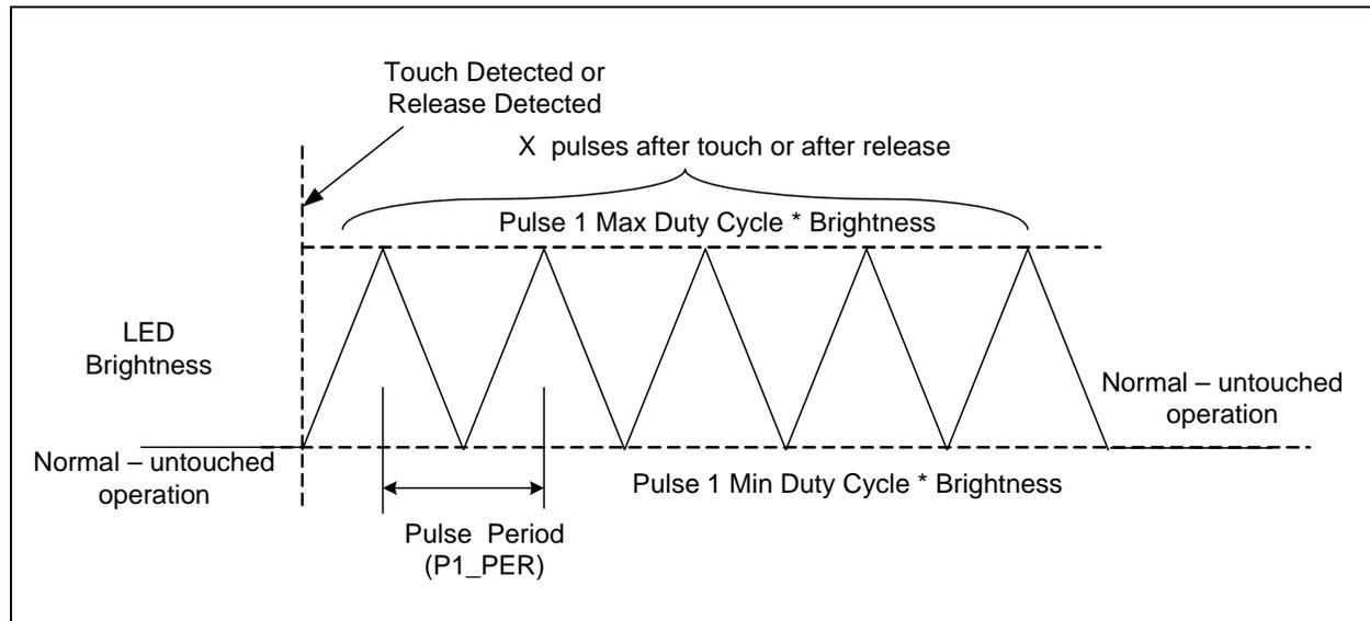
Figure 5.2 Pulse 1 Behavior with Inverted Polarity
