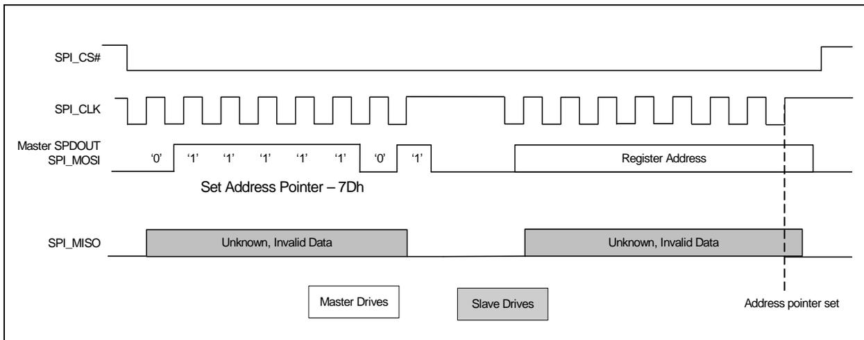
Figure 3.5 SPI Set Address Pointer Command - Normal Mode
