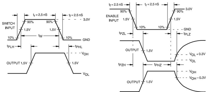
FIGURE 3. AC Waveforms
