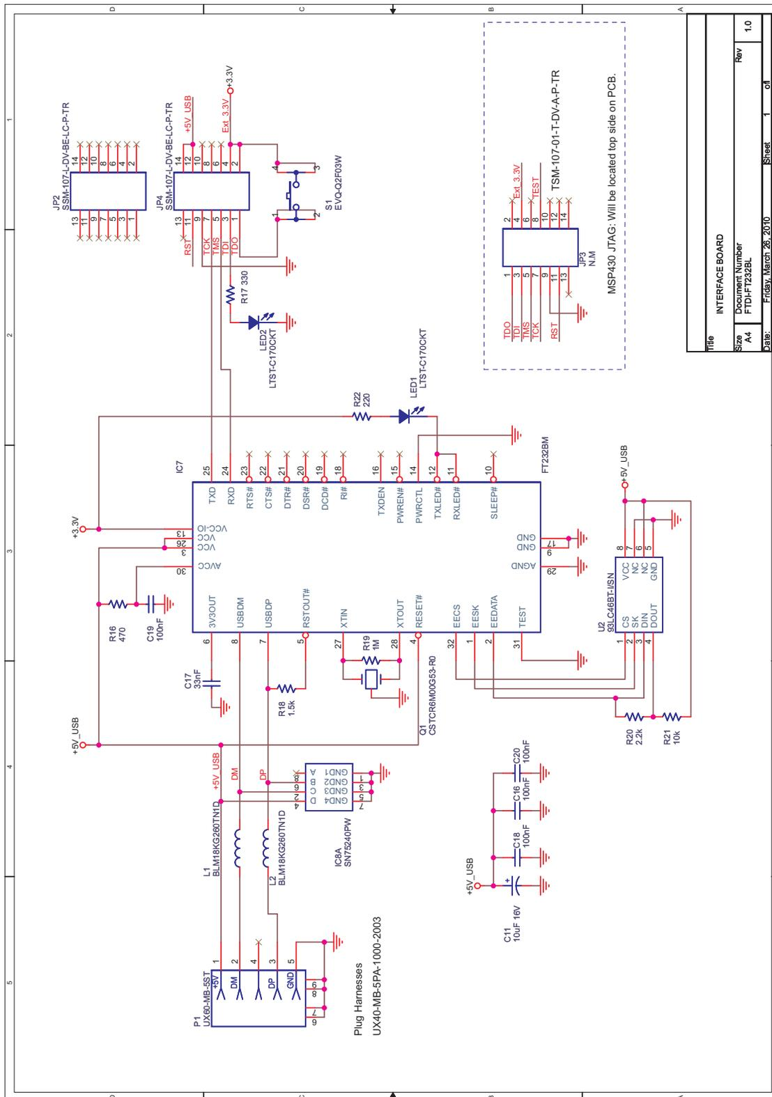
Figure 45. RFID Base Station Interface Board Schematic
