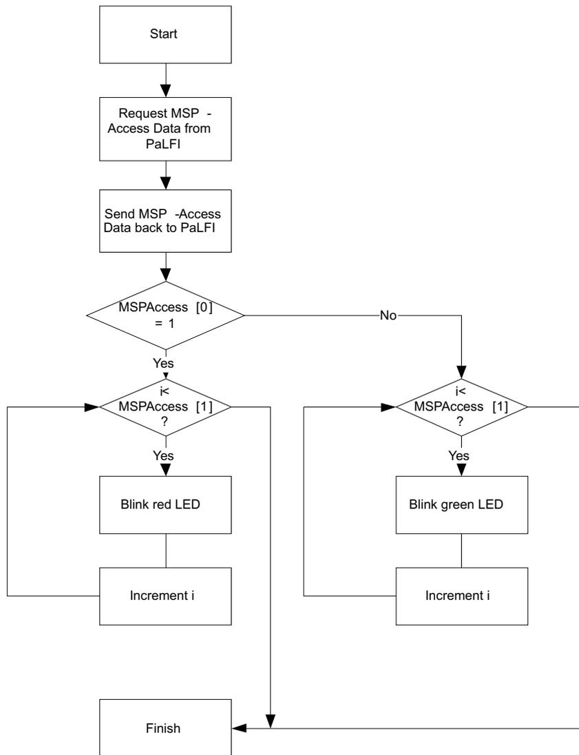
**Figure 33. Flow Diagram of MSP Access Routine**
