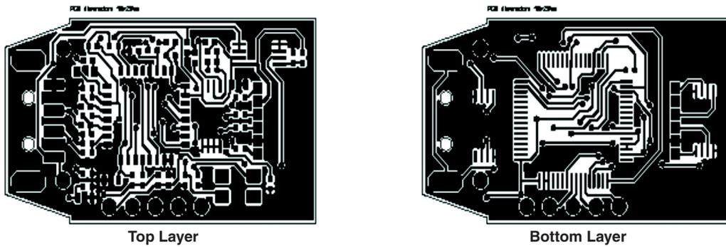
Figure 41. eZ430-RF USB Debugging Interface, PCB Layout
