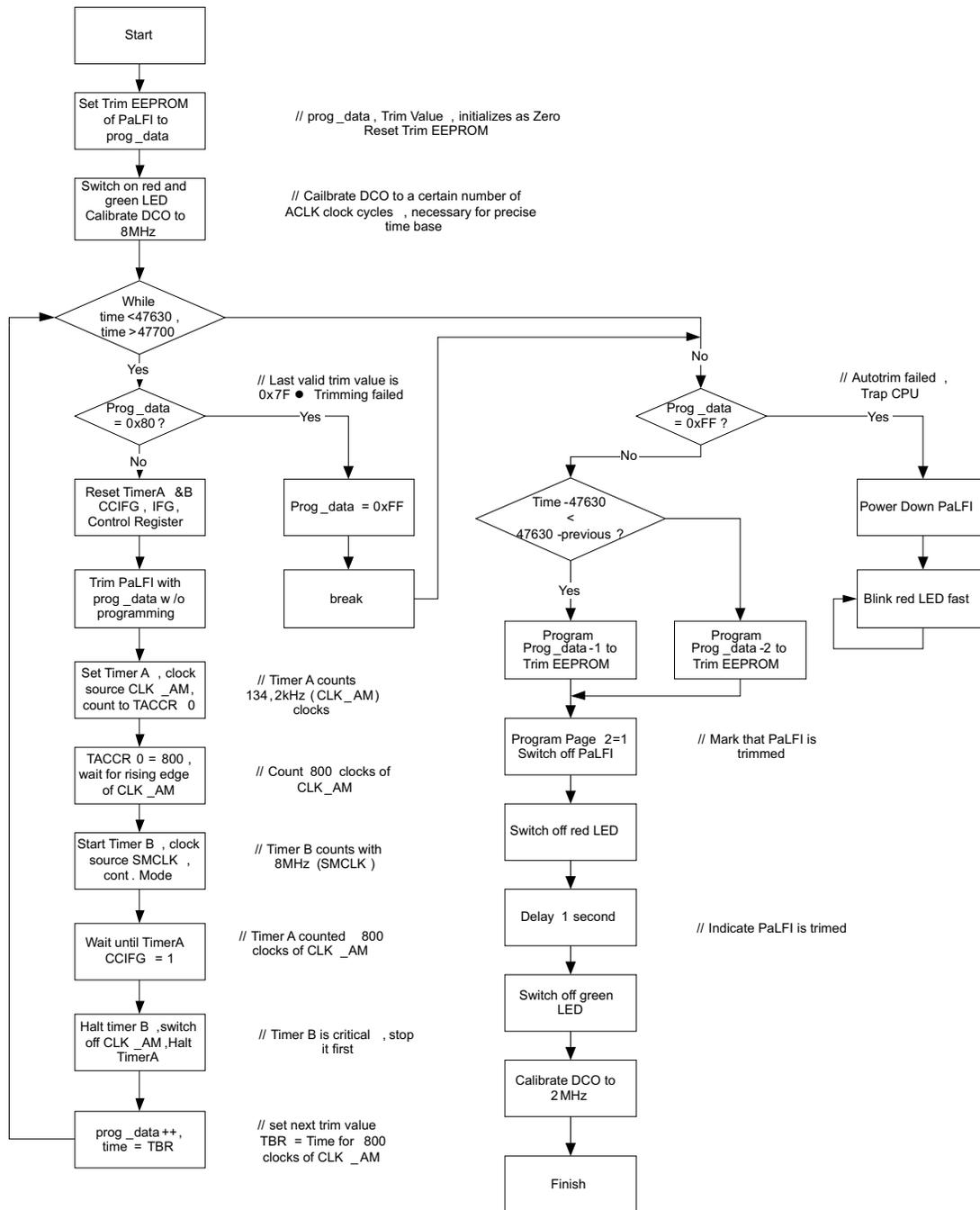
Figure 34. Flow Diagram of Auto Trim Routine
