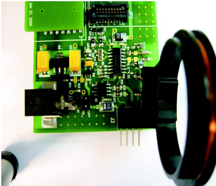
**Figure 4. RFID Base Station With Mounted Antenna**
