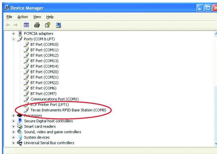
Figure 11. RFID Base Station in Device Manager
