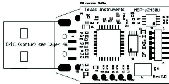
Figure 40. eZ430-RF USB Debugging Interface, PCB Components Layout
