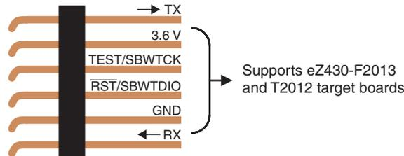
**Figure 35. eZ430-RF2500 USB Debugging Interface 6-Pin Male Header**
