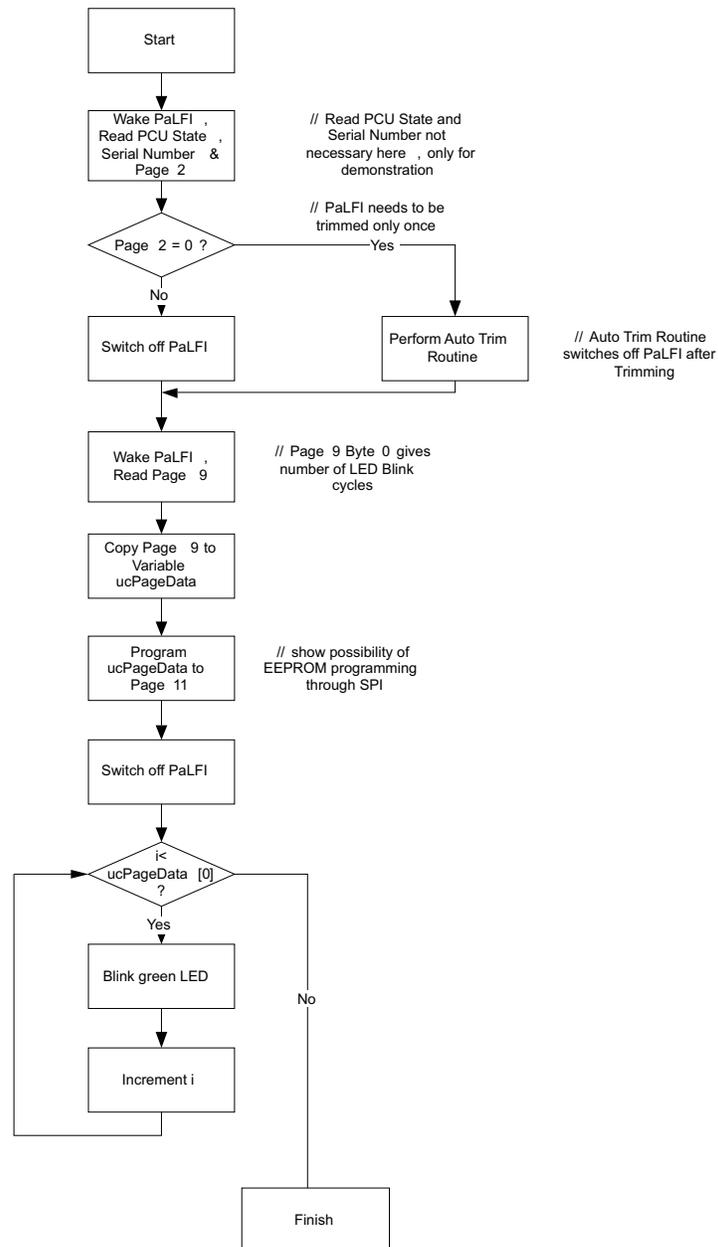
**Figure 32. Flow Diagram of Push Button Routine**
