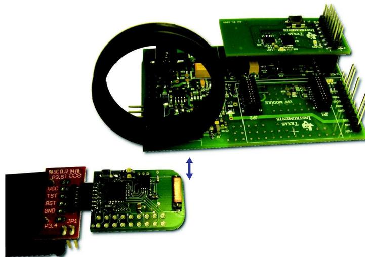
Figure 13. eZ430-TMS37157 in Front of RFID Base Station
