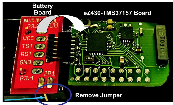
Figure 12. Connection of TMS37157 to the Battery Board
