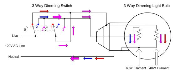
Figure 2.2: Three way dimming filament lamp system
