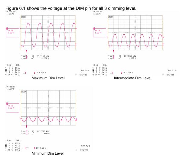
Figure 6.1: IRS2530D DIM pin voltages
