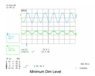
Figure 6.3: Lamp Voltage and Arc Current
