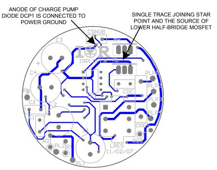
Figure 8.2: Critical traces on the top side of the PCB
