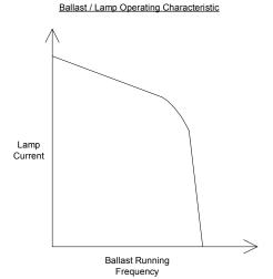
Figure 2.3: Lamp current against ballast frequency
