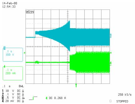
Figure 6.4: Lamp Voltage and Arc Current during preheat and ignition
