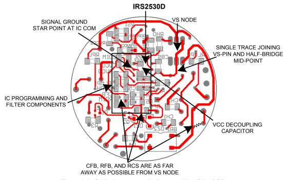
Figure 8.1: Critical traces on the bottom side of the PCB
