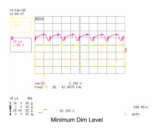
Figure 6.2: IRS2530D VCO (red) and VS (yellow) pin voltages
