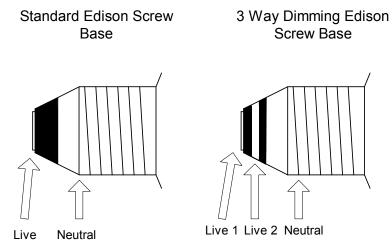
Figure 2.1: Three way dimming Edison screw base
