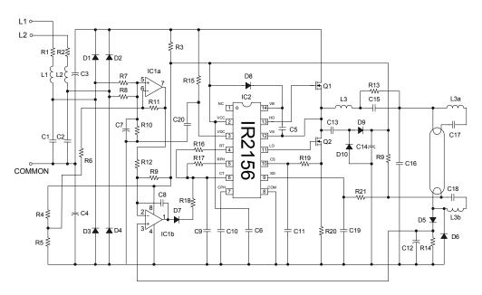
Figure 2.5: IRPLCFL4 Circuit Schematic
