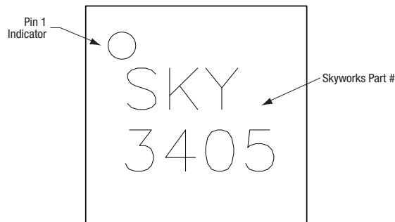
Figure 9. Typical Part Markings (Top View)
