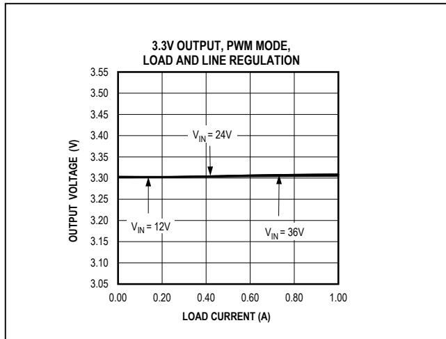
Figure 1. MAX17542G 3.3V Output Load and Line Regulation
