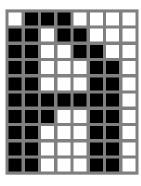
To allow for graphic block, all bits of each byte are used. In the default font B0 of each byte is used as space.
