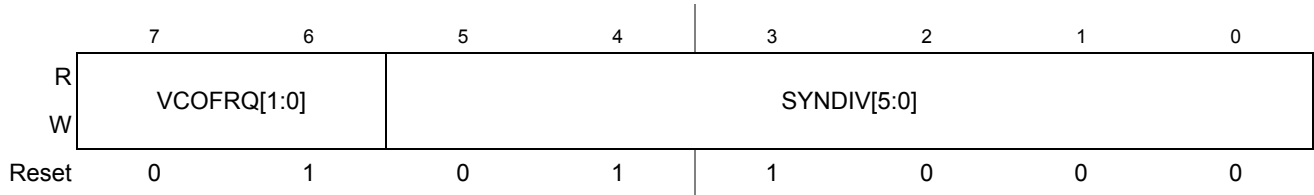
Figure 7-5. S12CPMU_UHV_V5 Synthesizer Register (CPMUSYNR)
