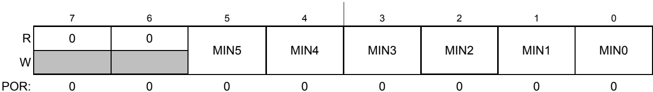
Figure 18-11. Minute Register (MINR)
