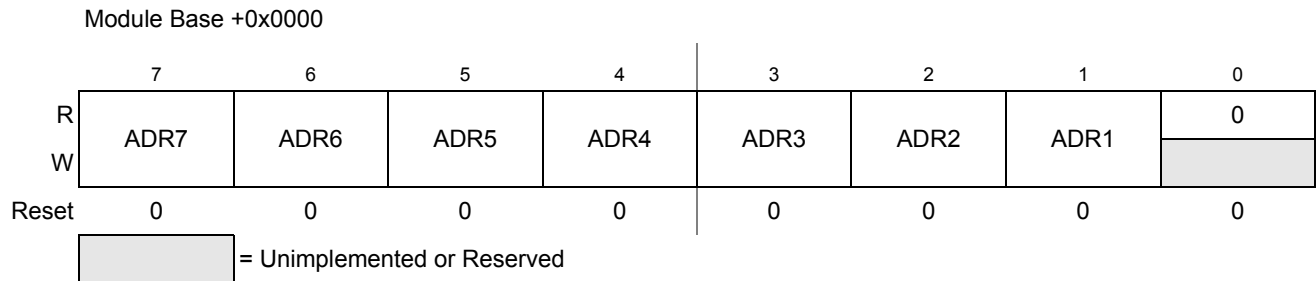
Figure 14-3. IIC Bus Address Register (IBAD)
