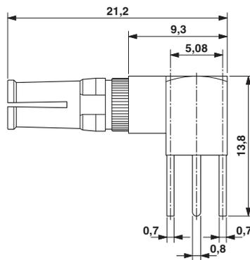
D-SUB coaxial contact pin
