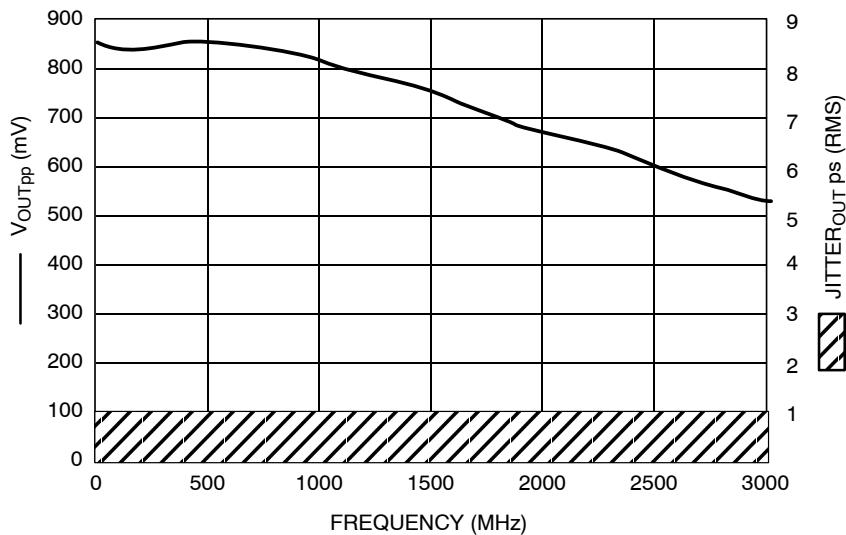
Figure 4.  $F_{max}$ /Jitter for QHG,  $\bar{Q}HG$  Output
