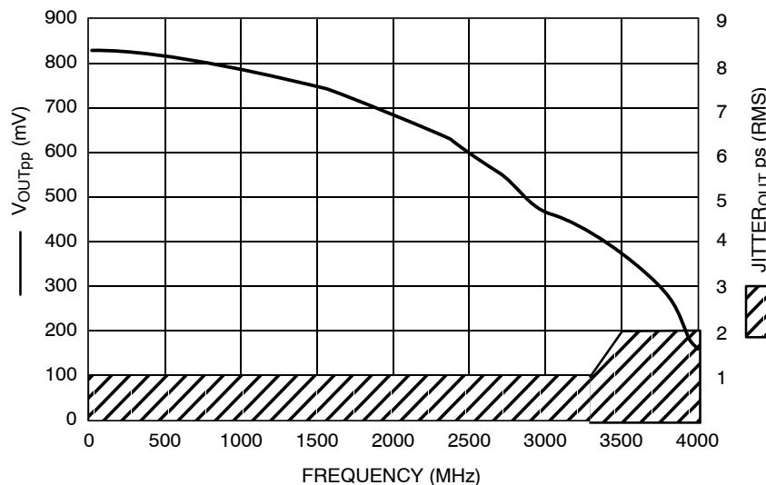
**Figure 2.  $F_{max}$ /Jitter for QHG, QHG Output**
