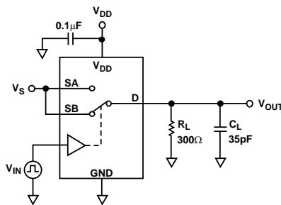
Figure 14. Break-Before-Make Time Delay,  $t_D$
