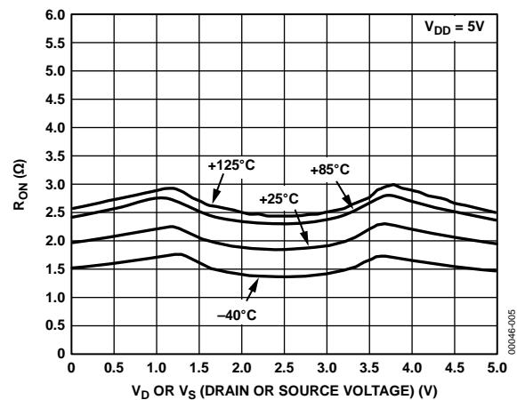
Figure 5. On Resistance as a Function of  $V_D$  or  $V_S$  for Different Temperatures
