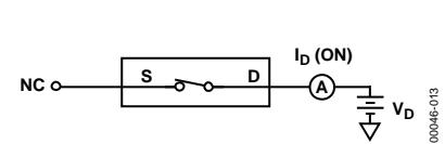
Figure 12. On Leakage
