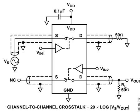
Figure 16. Channel-to-Channel Crosstalk
