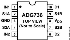
Figure 2. Pin Configuration
