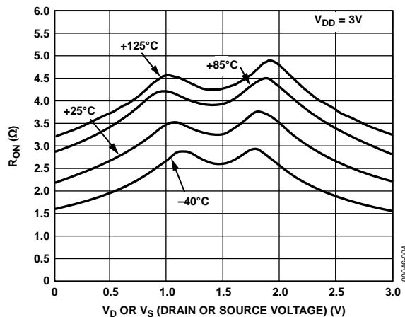
Figure 4. On Resistance as a Function of  $V_D$  or  $V_S$  for Different Temperatures
