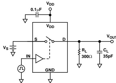
Figure 13. Switching Times
