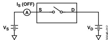
Figure 11. Off Leakage
