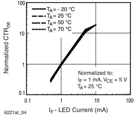
Fig. 4 - Normalized  $CTR_{ce}$  vs. LED Current
