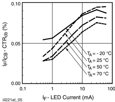
Fig. 5 - CTR<sub>CE</sub> vs. LED Current
