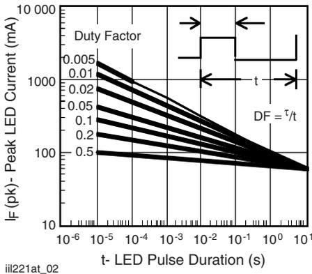
Fig. 2 - Peak LED Current vs. Duty Factor,  $\tau$
