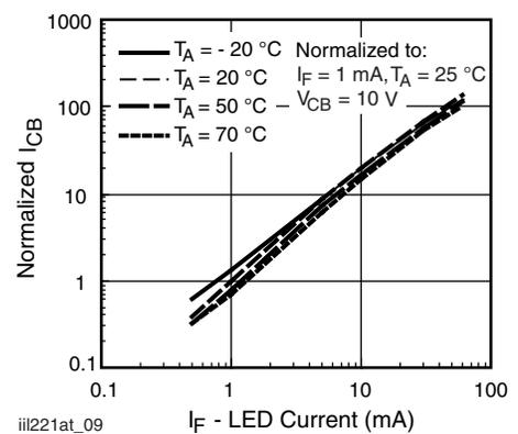
Fig. 9 - Normalized I<sub>CB</sub> vs. I<sub>F</sub>
