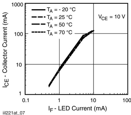
Fig. 7 - Collector Current vs. LED Current
