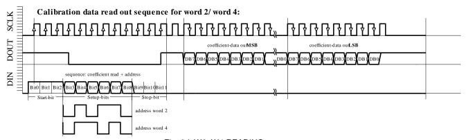
Fig. 6d: W2, W4 READING sequence
