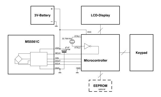
Figure 7: Demonstration of MS5561C in a mobile altimeter
