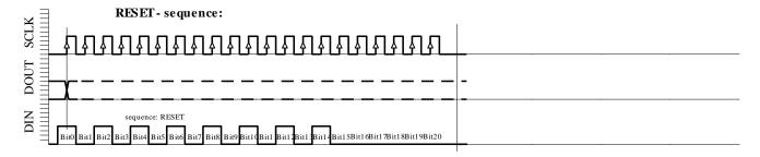
Fig. 6e: RESET sequence (21 bit)
