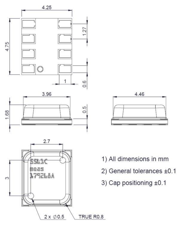
Fig. 8: Device package outlines of MS5561-C
