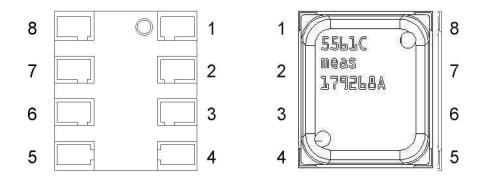
Fig. 2: Pin configuration of MS5561C
