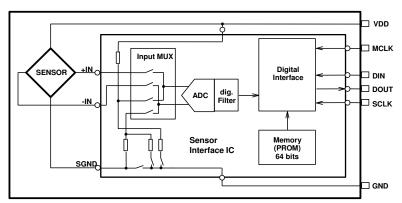
Fig. 1: Block diagram MS5561C
