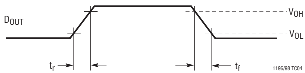
Voltage Waveform for D_{OUT} Rise and Fall Times, t_r , t_f
