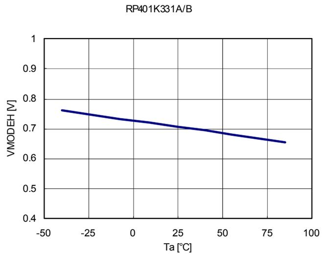
16) Output voltage vs. Temperature
