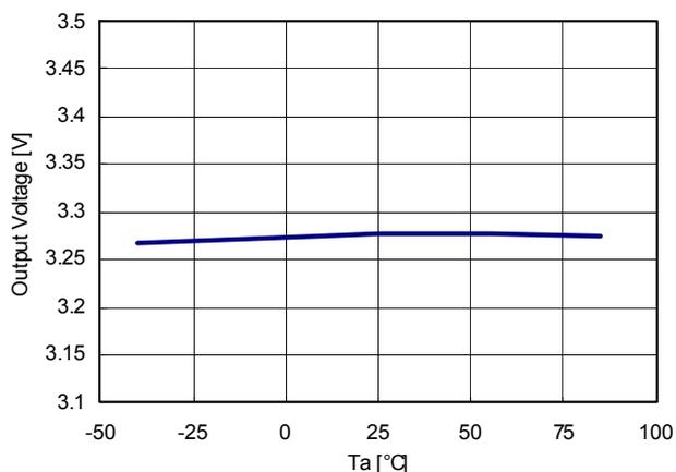
17) Feedback voltage vs. Temperature
