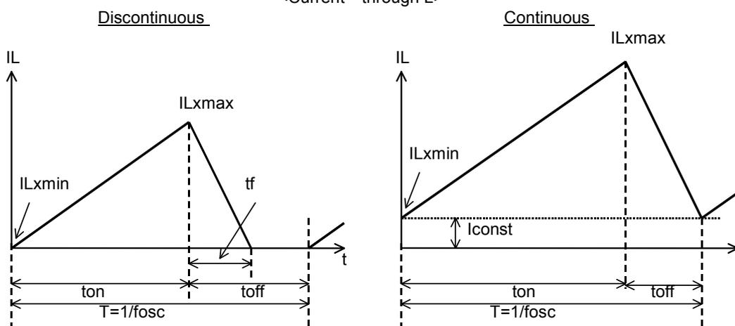
There are two modes, or discontinuous mode and continuous mode for the PWM step-up switching regulator depending on the continuous characteristic of inductor current. During on time of the transistor, when the voltage added on to the inductor is described as  $V_{IN}$ , the current is  $V_{IN} \times t / L$ .
