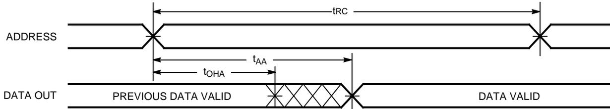
Figure 5. Read Cycle No. 2 ( $\overline{OE}$  Controlled)<sup>[12, 13]</sup>
