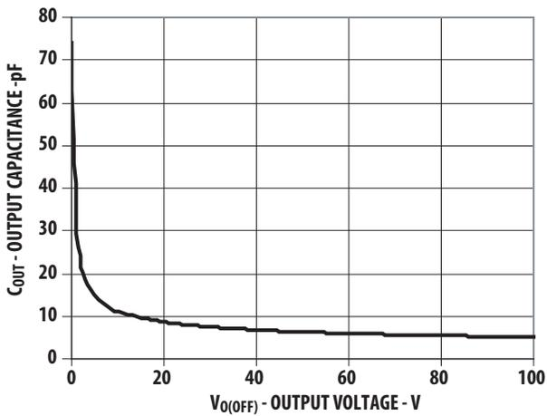
Figure 15. Typical Output Off-State Capacitance vs Output Voltage
