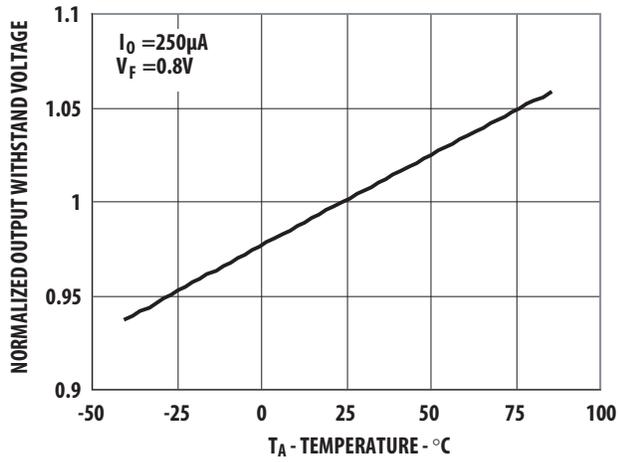
Figure 5. Normalized Typical Output Withstand Voltage vs. Temperature
