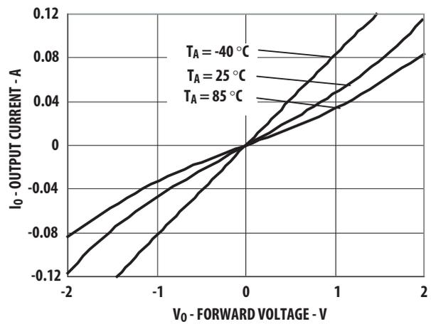
Figure 10. Typical Output Current vs. Output Voltage
