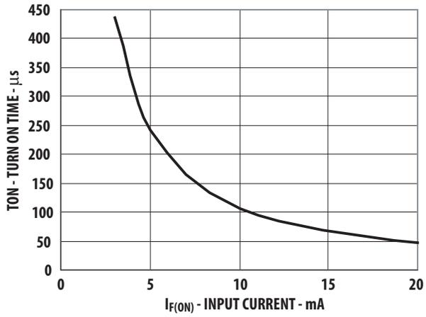
Figure 11. Typical Turn On Time vs. Input Current
