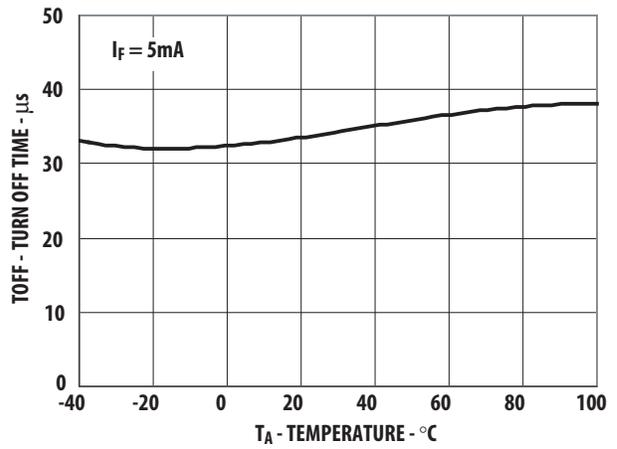
Figure 14. Typical Turn Off Time vs. Temperature
