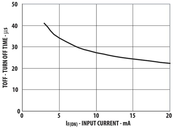
Figure 13. Typical Turn Off Time vs. Input Current
