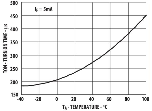
Figure 12. Typical Turn On Time vs. Temperature
