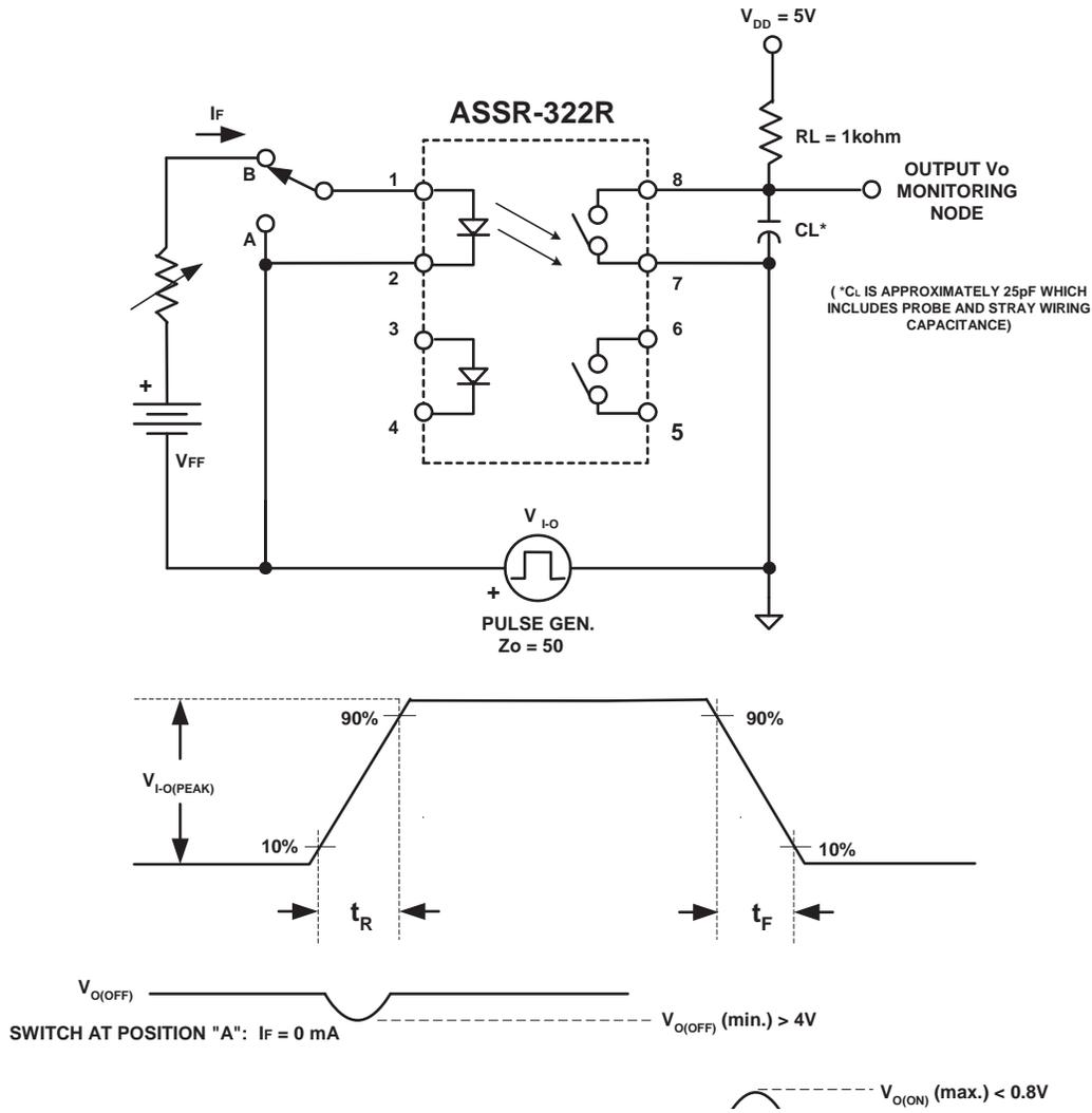
Figure 16. Switching Test circuit for  $t_{ON}$ ,  $t_{OFF}$
