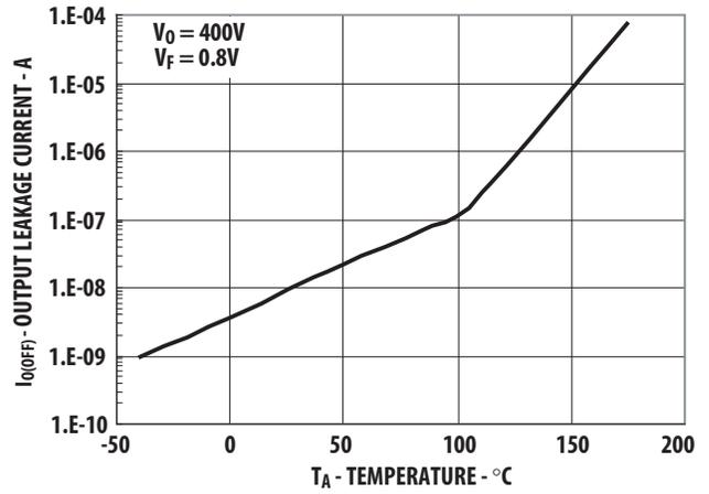
Figure 6. Typical Output Leakage Current vs. Temperature
