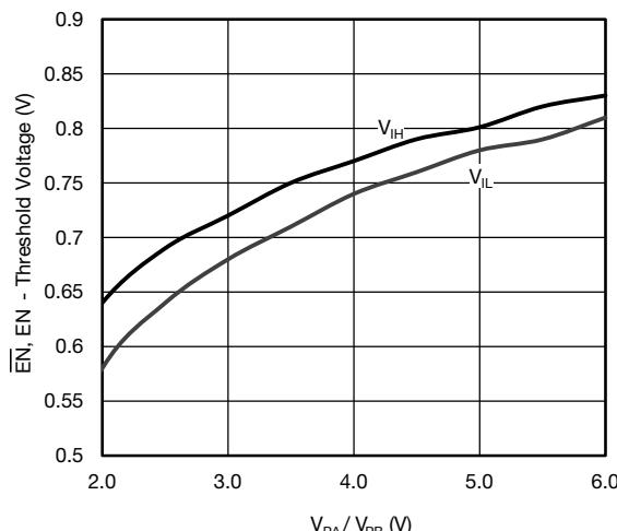
**Fig. 15 -  $\overline{E}N, EN$  Threshold Voltage vs. Input Voltage**
