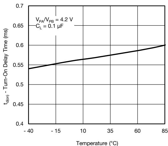
**Fig. 16 - Turn-on Delay Time vs. Temperature**
