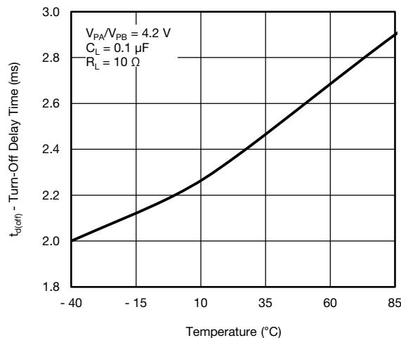
**Fig. 17 - Turn-off Delay Time vs. Temperature**
