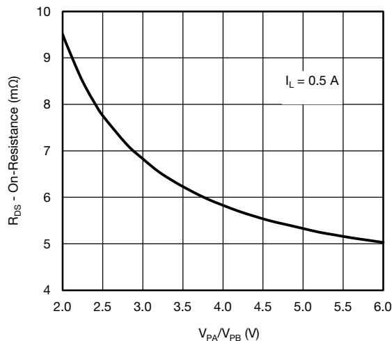
**Fig. 10 - On Resistance vs. Input Voltage**
