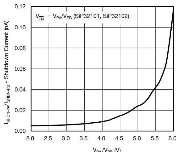
**Fig. 5 - Shutdown Current vs. Input Voltage**
