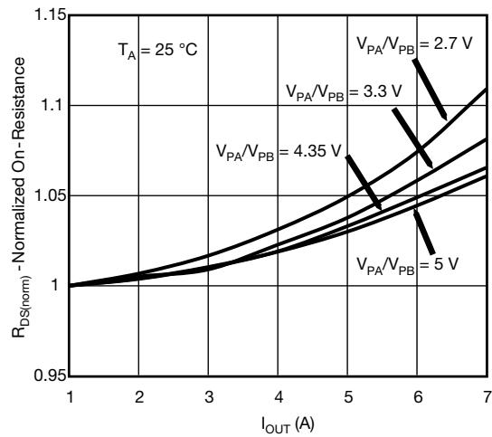
**Fig. 12 - Normalized On Resistance vs. Load Current**
