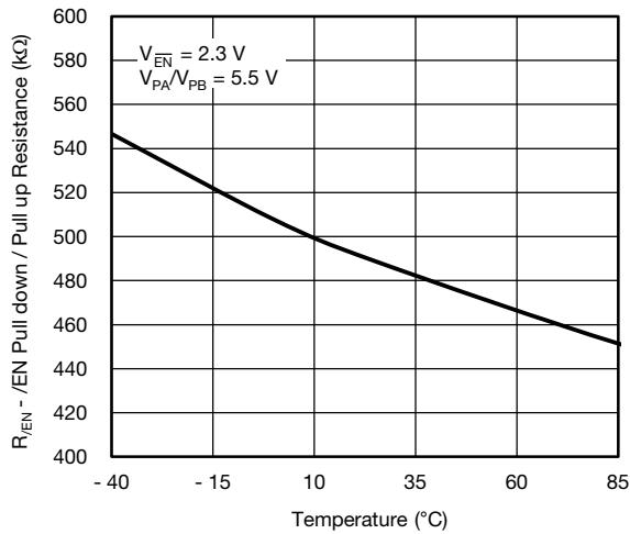
**Fig. 11 - EN Pull down Resistance vs. Temperature**
