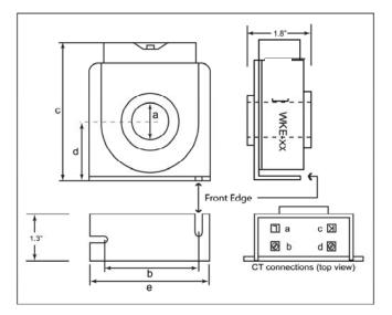
**Primary Current** 2500A **Secondary Current** 350mA NSV 600Vac **BIL Rating** 2000V **Rated Frequency** 10 – 1000Hz 70° C Thermal current rating **No Fixed Burden** 99% Accuracy Flux Shielding
