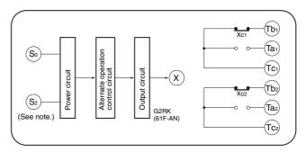
$\left( \begin{array}{c} \textbf{Note:} \text{ The above diagram is for a rated voltage of 200 or 220 VAC.} \\ \text{Power is supplied to $S_0$ and $S_1$ for 100 or 110 VAC.} \\ \text{Connections (Refer to connection diagram.)} \end{array} \right)$
