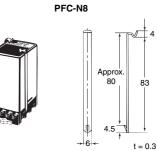
Note: PFC-N8 Mounting Bracket (provided with the Level Controller)
