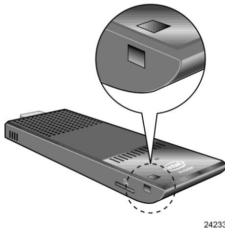
Figure 9. Security Loop Opening
