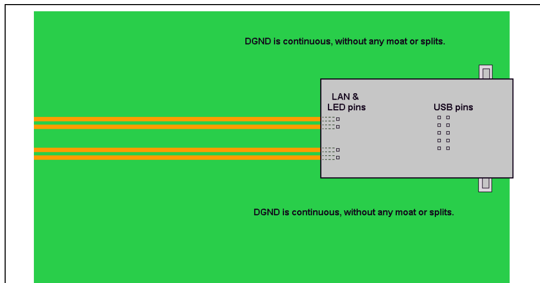
Figure 16-20. Ground Layout with USB
