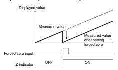
Press the Up Key while the measurement is being displayed. The displayed value will be shifted to 0 and measurement will be continued.
