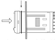
Fit the adaptor into the grooves on the left and right sides of the rear case, then push it until it contacts the panel to secure the K3MA-J.
