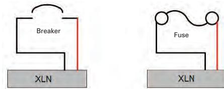
The XLN series can be used to accurately measure the time for a fuse or circuit breaker to open. After the voltage and current levels are set, the ON/OFF button turns on the output and the time when the fuse/breaker opens is measured to the nearest 100  $\mu$ s. The maximum counting period is one hour.
