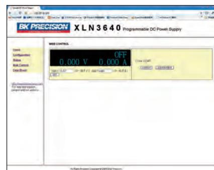
Interface for controlling voltage, current and output state
