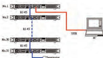
In multi-unit control mode, up to 31 units can be daisy chained via RS485 and controlled from one "master" unit via the USB interface (also GPIB and Ethernet).
