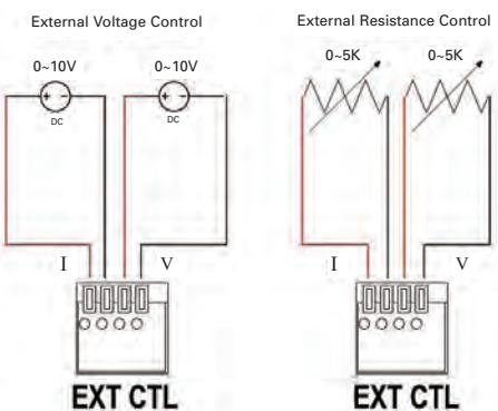
The output voltage and current can be controlled by either analog voltages or resistances. 0-10 V voltages and 0-5 k $\Omega$  resistances control from zero to full scale output.
