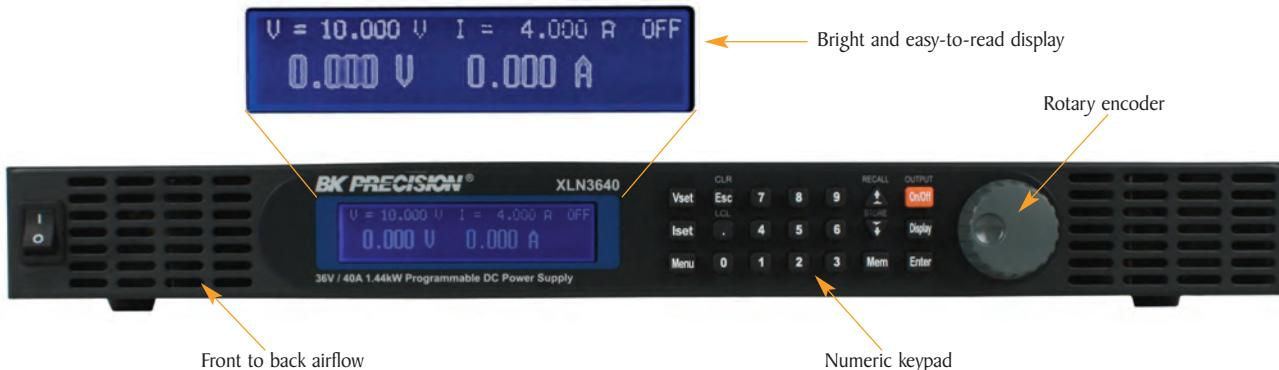
The numeric keys and rotary knob provide a convenient interface for setting output levels quickly and precisely. Voltage and current can be set to a maximum resolution of 1 mV and 1 mA, respectively. Both meter values (measured output
