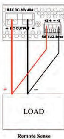
The remote sense feature can compensate for up to 2 volts of voltage drop in the load wiring. Two small wires connect to the +S and -S sense terminals (high input impedance) and the power supply changes its output to make the voltage on these sense lines equal to the voltage set on the front panel.
