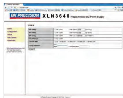
Setting Controls page for configuration of protection settings and setup/reset password for the system.
